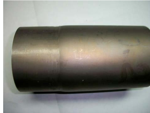
Fig. 2: A thin-walled precision pipe with a diameter D = 80 mm with wall thickness t = 0.8 mm from PT-7M titanium alloy with calibrated end by the squeezing mode
