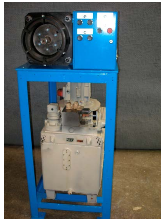
Fig. 6: Installation for calibration of the ends of thin-walled pipes
