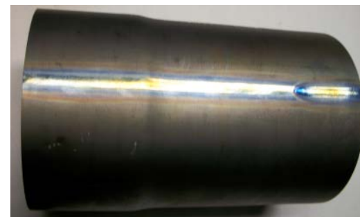
Fig. 3: A thin-walled precision pipe with a diameter D = 100 mm with wall thickness t = 0.8 mm from VT1-0 titanium alloy with calibrated end by the expanding mode
