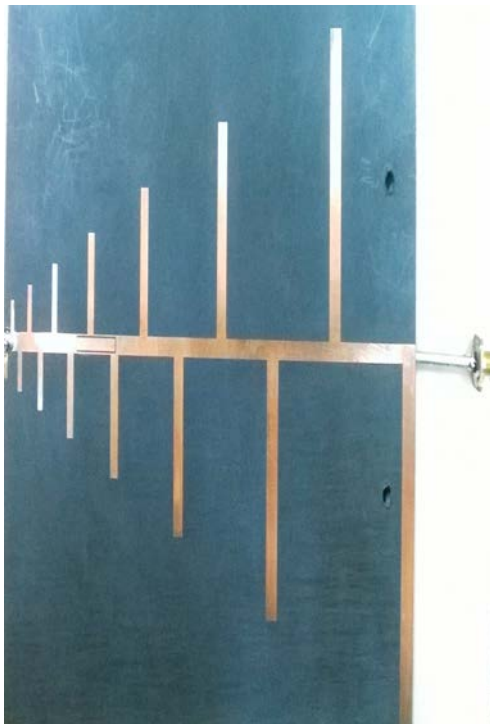
Fig. 2: Fabricated PLPDA with notched filter
