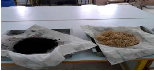
Fig. 2: Treated pumice and limestone cubes after crushing
