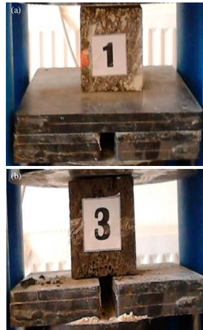
Fig. 1: Limestone and pumice cubes after treating: a) treated limestone cubes and b) treated pumice cubes
