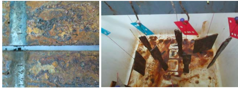
Fig. 2: Corroded plates in salt spray machine
