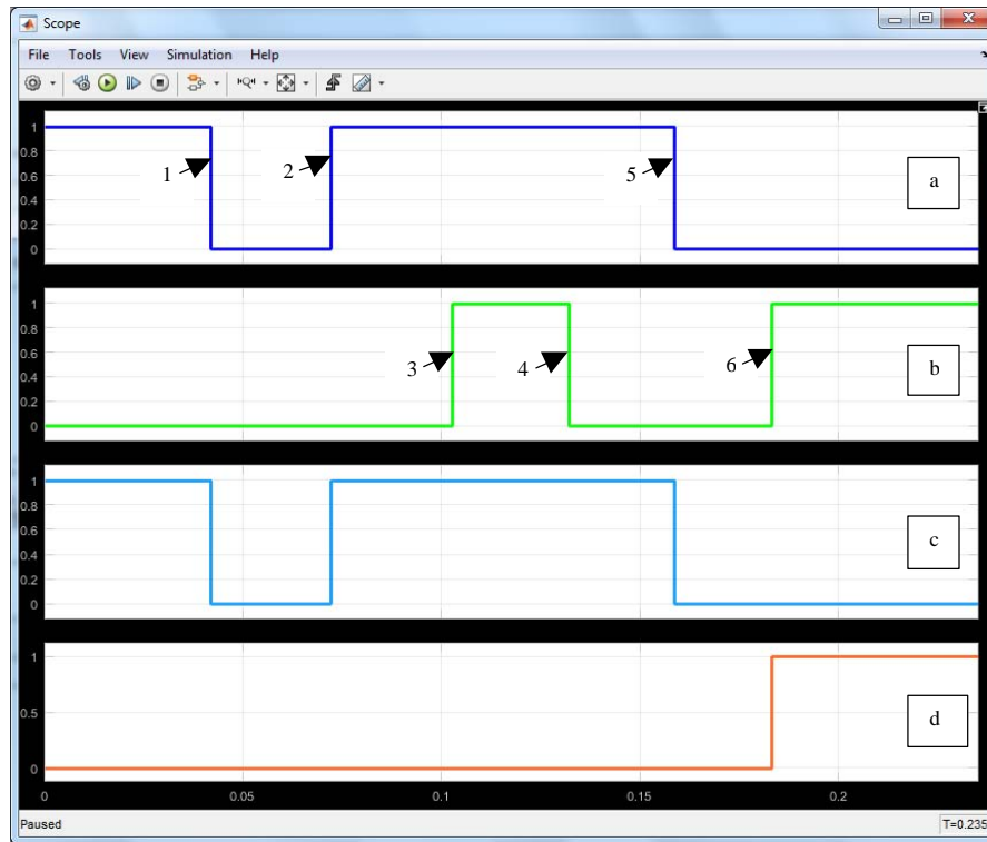
Fig. 6: Signal diagrams in blocking scheme: a) command to main blades closing; b) command to earthing switches closing; c) control signal of main blades and d) control signal of earthing switches
