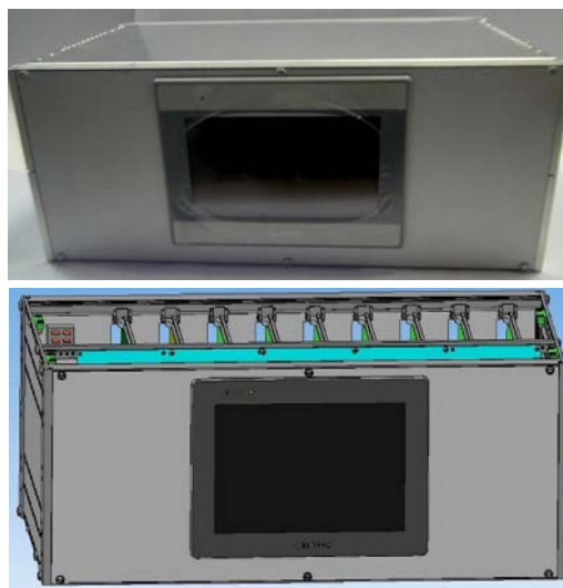
Fig. 1: Appearance (above) and a computer model in COMPASS (below) of the breadboard for smart relay protection of electrical networks
