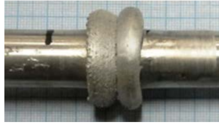
Fig. 3: Without chamfer angle ( 0^\circ ), surface roughness of 1.0667 \mu\text{m}
