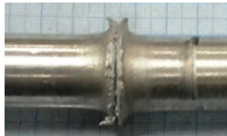
Fig. 5: Chamfer angle of 15^\circ , surface roughness of 1.0667 \mu\text{m}
