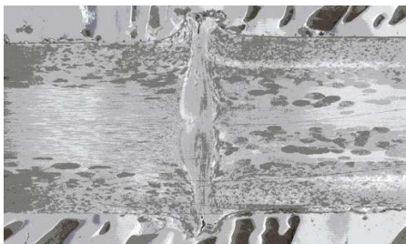
Fig. 10: Chamfer angle of 15°, surface roughness of 0.697 μm
