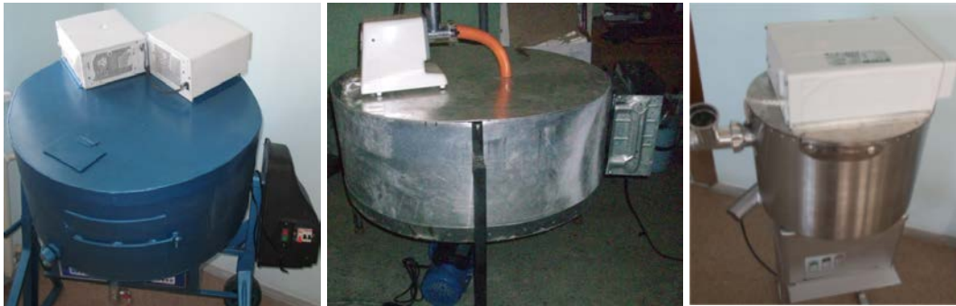
Fig. 9: Basic models of installations for heat treatment of fat-containing raw materials using electromagnetic radiation energy: a) Microwave and ultrasonic unit for fat-containing raw materials processing; b) Microwave installation for thermal treatment of fat-containing raw materials and c) Microwave installation for thermal treatment of fat
