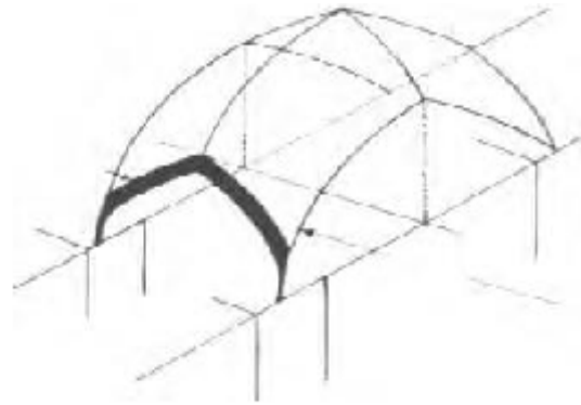
Fig. 9: An example of Palanquin arch in palace of forty columns of Isfahan
