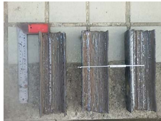
Fig. 6: Weld surface inside C-channel alloy steel
