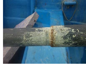
Crack at shaft shoulder
