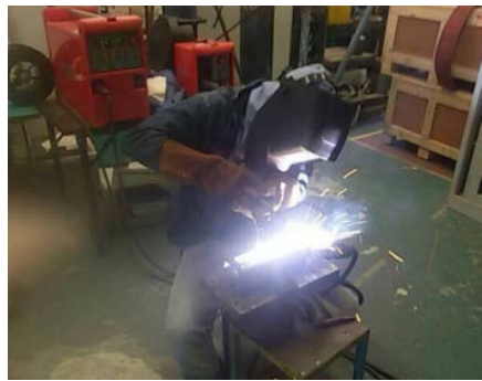
Fig. 7: Gas metal arc welding process and flux cored arc welding process which are semiautomatic welding process
