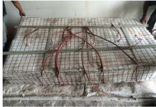
Fig. 1: Specially designed electrical furnace made up from ceramic fiber
