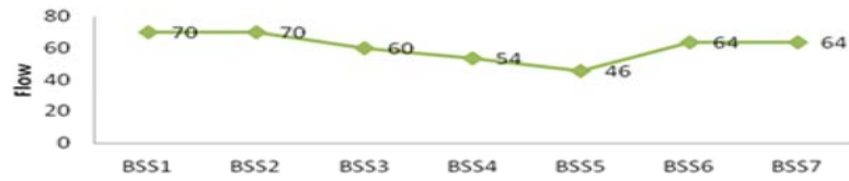
Fig. 7: Flow result for Bitumen-SBS-sulphur mixtures
