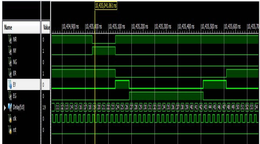
Fig. 9: North-East zones traffic clearance
