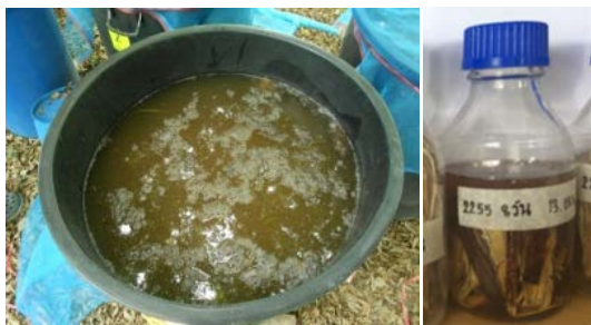
Fig. 1: a) Water retting: b) Chemical retting process
