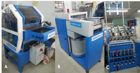
Fig. 2: Ring spinning process: a) Carding and waving; b) Sliver; c) Ring spinning
