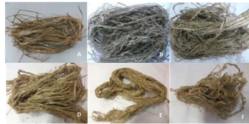
Fig. 4: Hemp fibre after water retting and chemical retting: a) Raw hemp bark; b) Water retting 1 week; c) Water retting 2 weeks; d) Water retting 4 weeks; e) Water retting 9 weeks; f) Chemical retting
