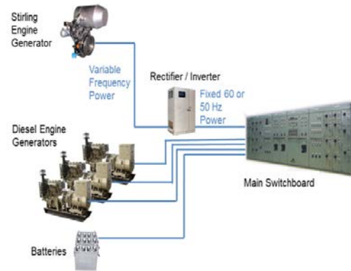
Fig. 6: Ship's electric power plant layout
