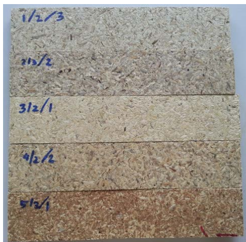
Fig. 3: Particleboard from core residue after testing A: KeR; B: KeM; C: HeM; D: HKM; E: HSD
