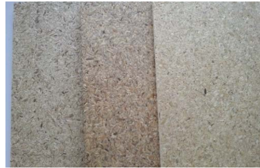
Fig. 4: Insulation board from core residue A: KeR; B: KeM; C: HeM
