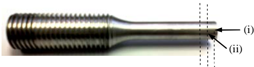
Fig. 5: Fatigue fracture surface indicates by (i) and the hardness test was performed about 2 mm under the fracture surface as indicated by (ii)
