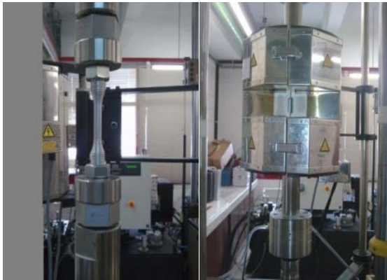
Fig. 4: Test set-up configuration for the cyclic test, (a) specimen attached to the machine and (b) specimen inside the heating chamber
