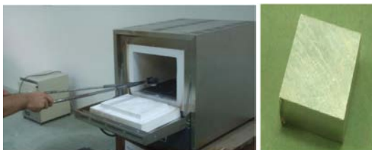
Fig. 15: The furance machine used for the third experiment on 300°C
