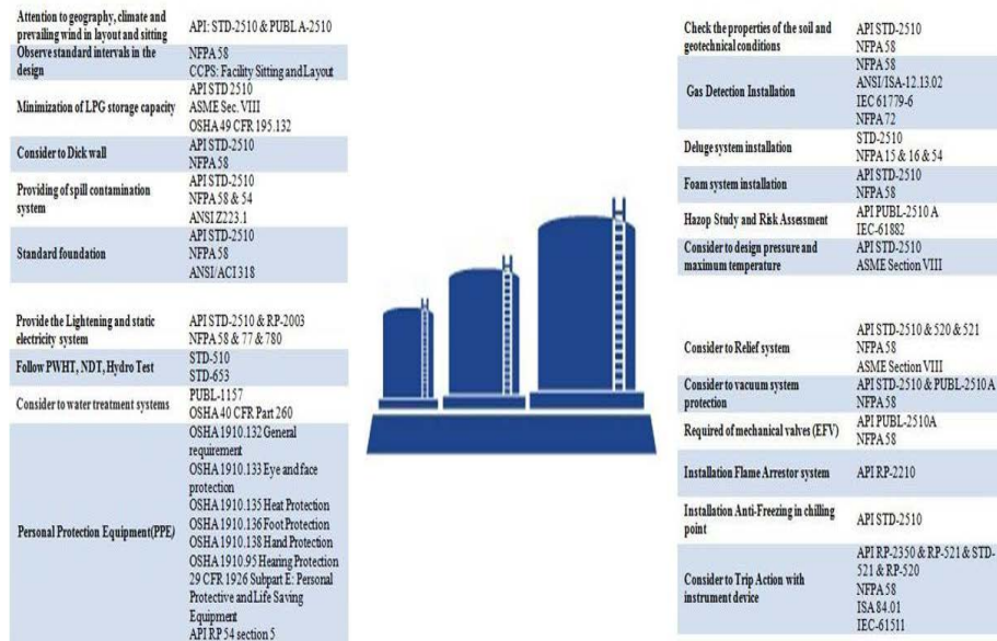
Fig. 7: LPG storage tank related standard
