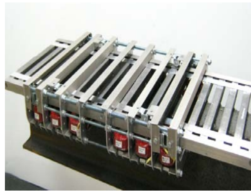
Fig. 7: Transports platform layout with magnetic suspension
