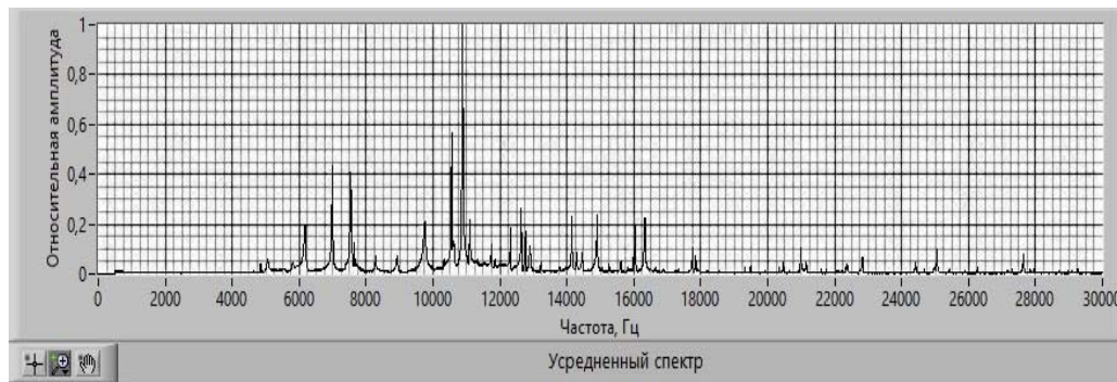
Fig. 7: TCR No. 4 defective case spectrum
