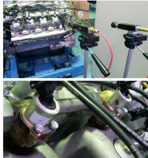
Fig. 10: Installation of laser vibrometers (on the left) and the location of a vibrometer laser beam pointing on gas dispensers (on the right)
