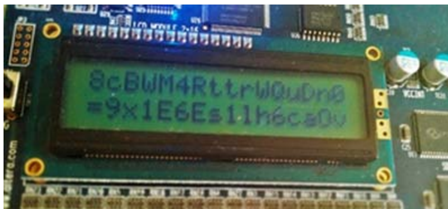
Fig. 8: The last 32 decoded characters
