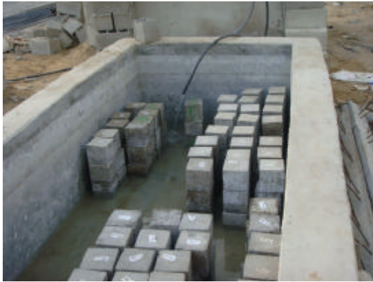
Fig. 4: Curing samples in a tidal environment
