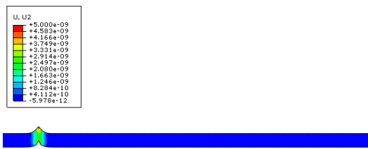
Fig. 24: Wave propagation condition of pulse stimulation in plane strain model at 1.5 \mu sec
