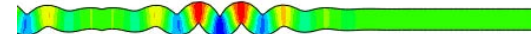
Fig. 15: Near operator wave propagation condition for A_0 stimulation mode by displacement at frequency of 600 \text{ kHz} at 54 \mu \text{ sec}
