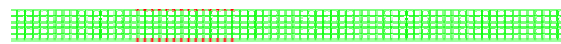
Fig. 28: Applied symmetric and asymmetric load nodes as lamb wave stimulation in wide stimulation model
