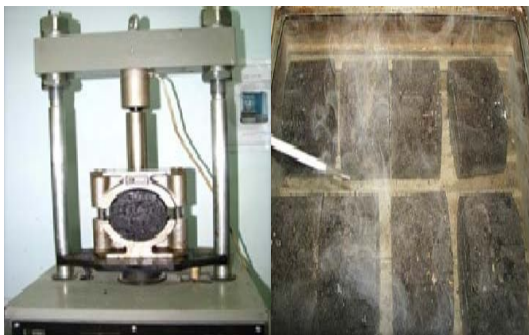
Fig. 4: Removing the mold test samples of actual specific gravity in a water bath
