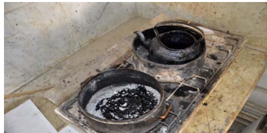
Fig. 6: The combination of materials, heating and preparation of asphalt
