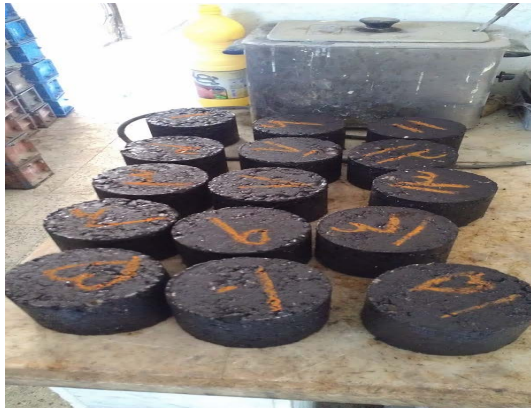
Fig. 9: Samples came out of asphalt bathroom
