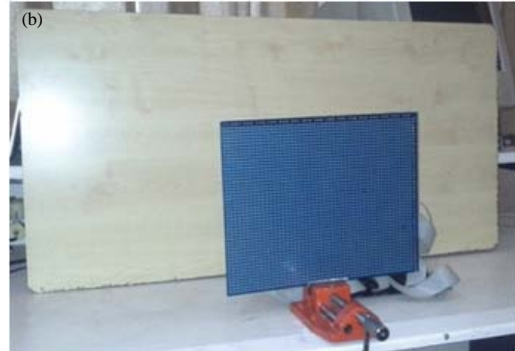
Fig. 9: a) Appearance of main resistance array and b) Placement of main resistance array in front of the camera
