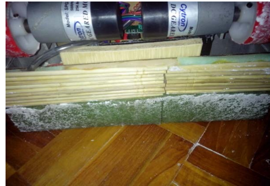
Fig. 11: Bottom surface with brush of the cleaner robot
