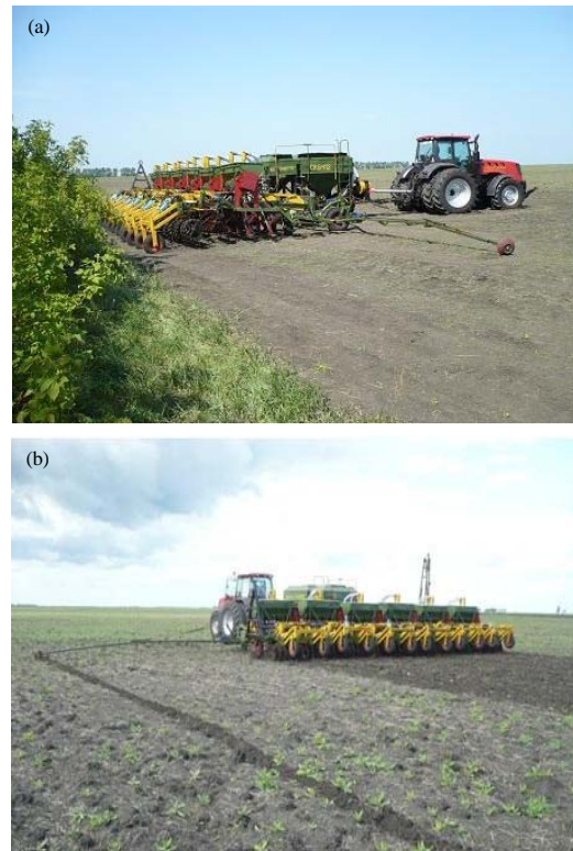
Fig. 3: Modular cultivator drill SKBM-12 with tractor belarus 3022DV; a) General view; b) In operating position
