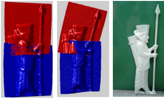
Fig. 10: Registration of achamenid soldier statue. Right image: color image of statue. middle image: two views of the statue before registration. left Image: 3D model of the statue after registration
