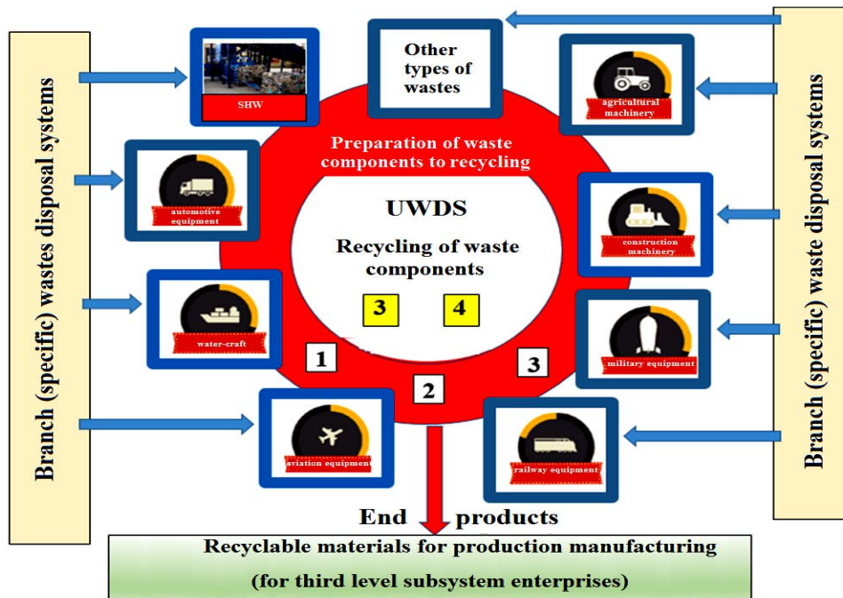
Fig. 5: Unified wastes disposal system structure
