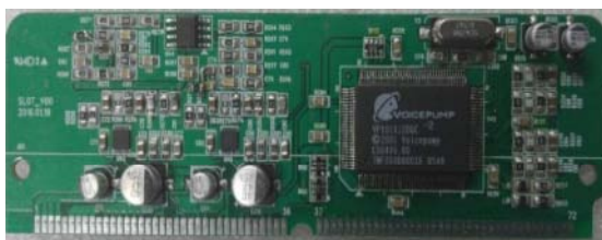
Fig. 9: The DSP board
