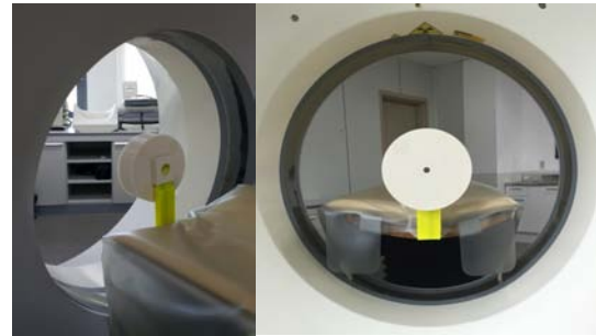
Fig. 4: Proposed CT phantom by 3D printing technology equipped at the CT scanner table-edge
