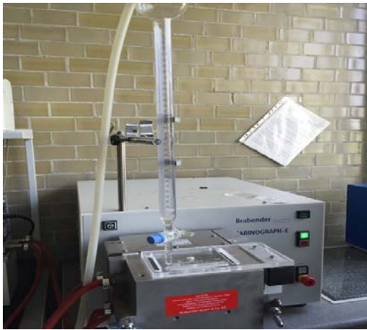
Fig. 1: The Farinograph instrument
