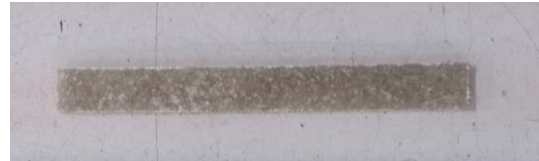
Fig. 4: A composite specimen for flexural bending test
