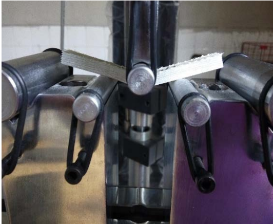
Fig. 9: Nanocomposite under the flexural bending test
