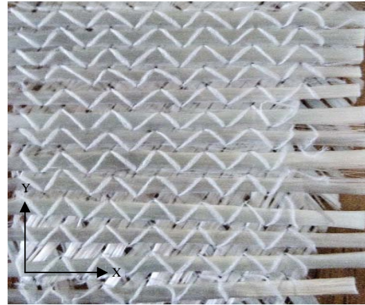
Fig. 1: The directions of X and Y in 3-directional glass fibers
