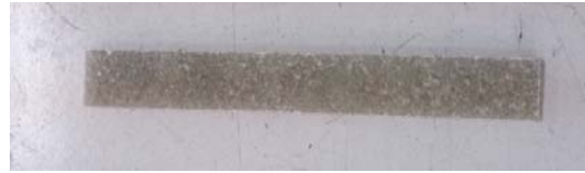
Fig. 3: Aspecimen for composite tensile test with dimensions of 120×15 mm
