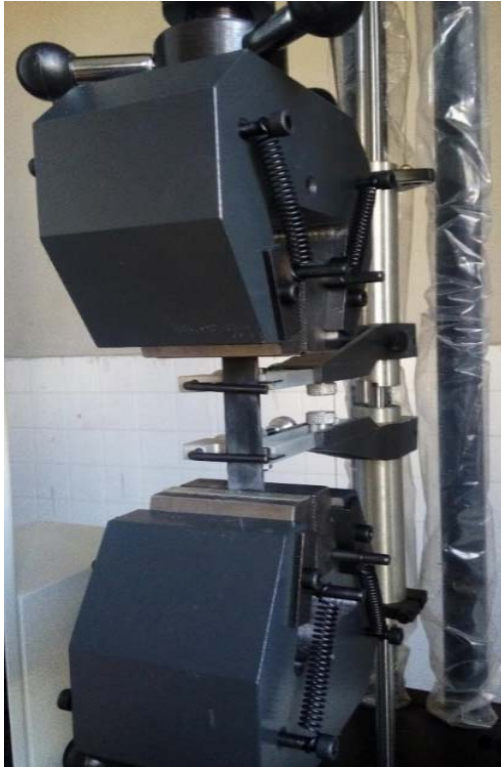
Fig. 6: Clay/nanocomposite during the tensile test
