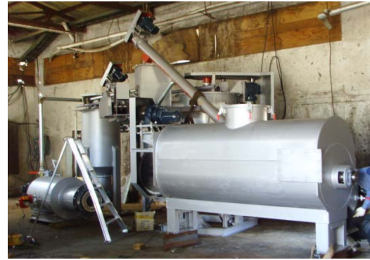
Fig. 4: Sample of a speedy dryer and thermal decomposition device
