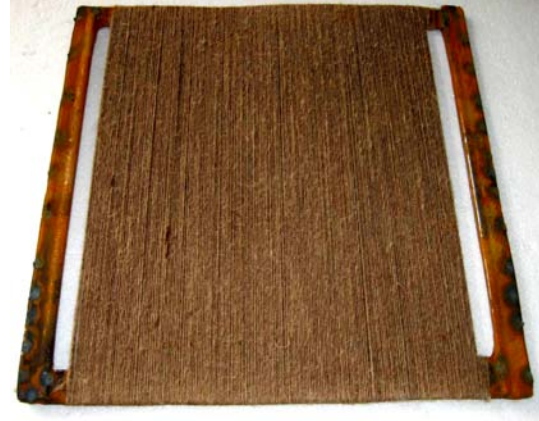
Fig. 1: Four layers of kenaf fiber woven around a steel frame
