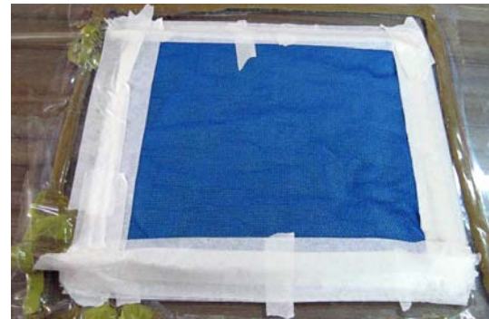
Fig. 2: Fabrication of specimen by VIP
