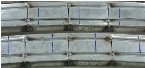
Fig. 4: The location of the weld at bottom flange and double intermediate web stiffeners
