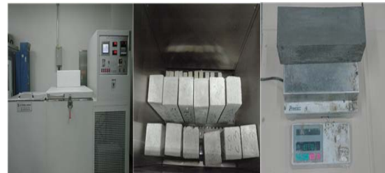
Fig. 2: Measurement test of freezing-thawing resistance
