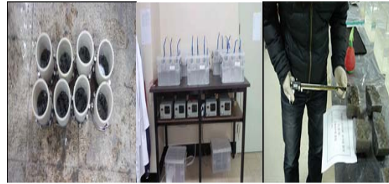
Fig. 1: Chloride diffusion coefficient measurement test
