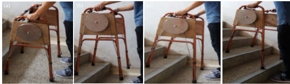
Fig. 1: Steps on ascending stairs: a) Hold the walker level on the ground; b) Carry it onto the first step; c) Exert a force downwards so the hind legs would elongate and d) Shift the weight of your leg forward with the handle support and repeat everything on the following steps
