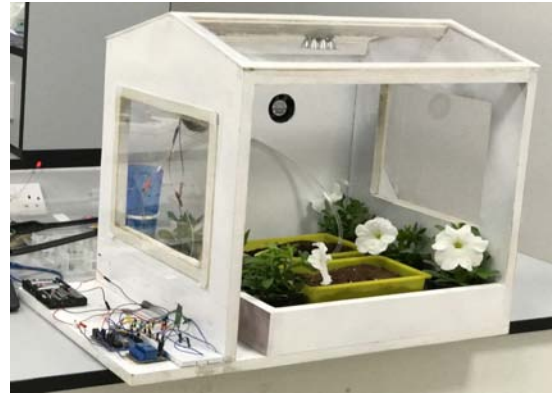
Fig. 5: Prototype green house automatic control system built in the laboratory
