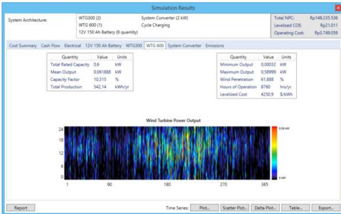
Fig. 12: Power output of the 600 W wind Turbine
