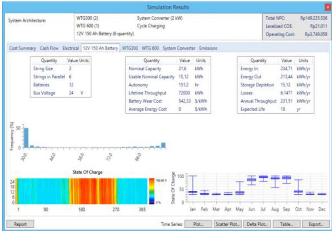
Fig. 10: State of charge of the battery system
