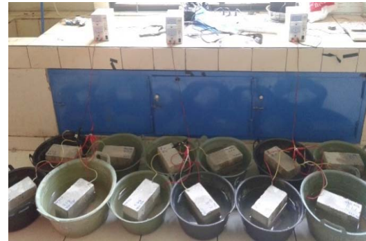
Fig. 2: Accelerated corrosion in laboratory
