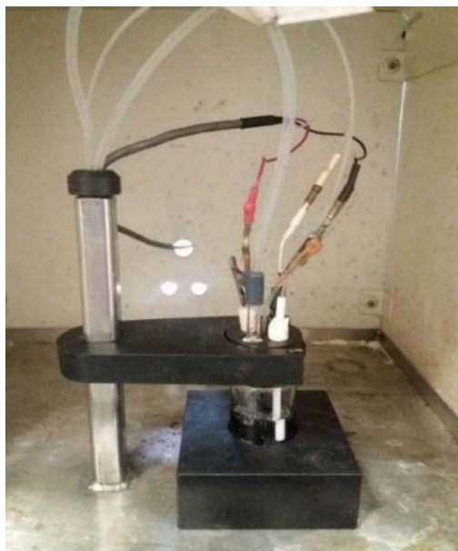
Fig. 2: Mounting of cell for polarization resistance test
