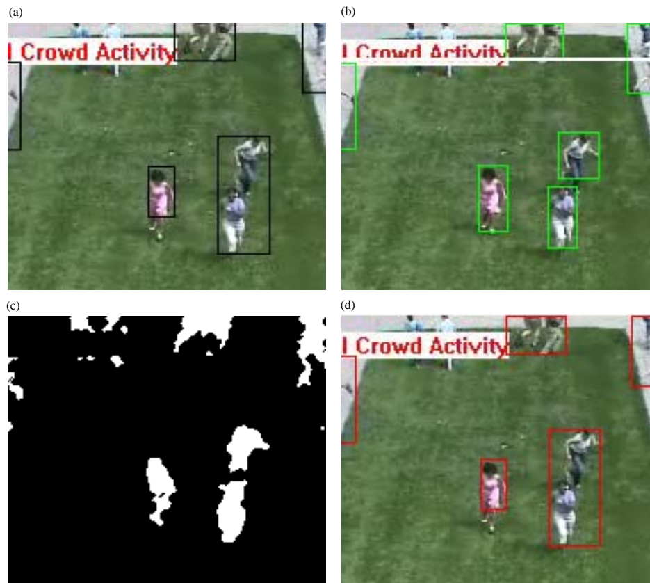
Fig. 4: a) Objects detected according to distance; b) Simple object detection; c) Threshold video and d) Objects detected according to velocity
