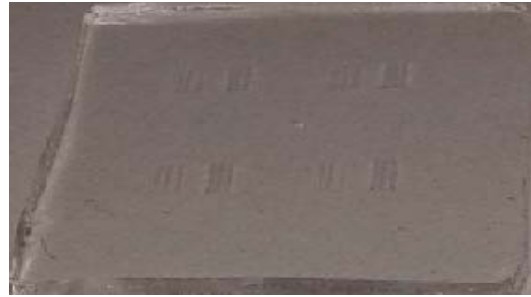
Fig. 6: PDMS printing plate with fine solid line image
