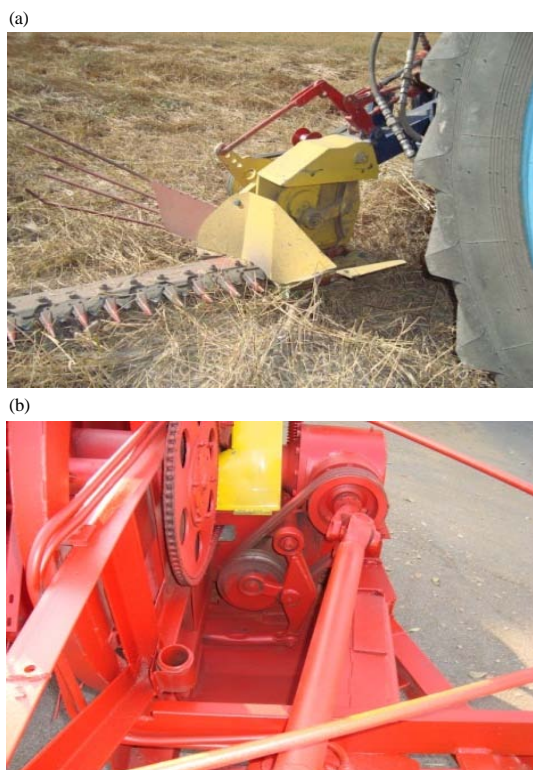
Fig. 9: a) Crank-rocker mechanisms for driver of the cutting device with a double stroke which are used in mowers and b) In mower-conditioner KP-3.0
