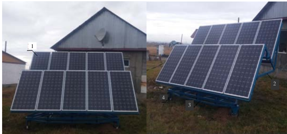
Fig. 2: The general view of SPM prototype during laboratory tests: 1) SP; 2) bearing frame; 3) main frame and 4) wheels
