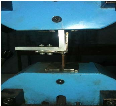
Fig. 18: Jig fixture of tensile tests
