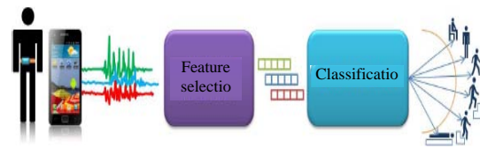
Fig. 3: Activity recognition process pipeline (Anguita et al. , 2012)
