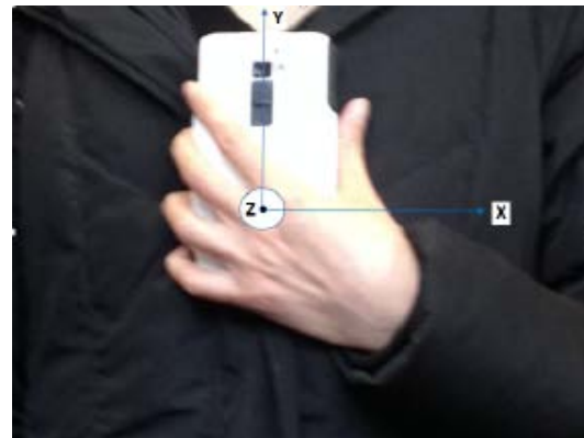
Fig. 1: Android smart phone with its axis direction for accelerometer (Bayat et al. , 2014)
